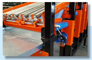
The PERFECT cherry sorting machine is standard supplied with a spindle system that changes the sorting diameter. The distance between the axles is set very precisely.
