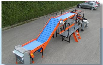
In order to reduce the load on the employees, an unloading platform with elevator is optionally available.
