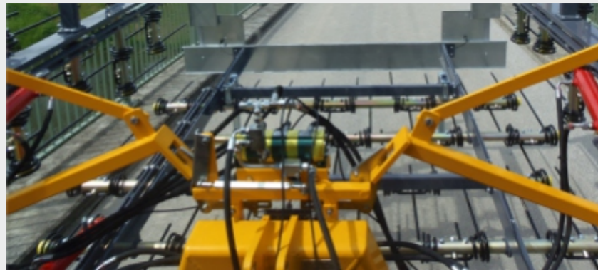
Standard with check valves on double-locking hydraulic cylinders. Optional protective cover for the teeth when driving on public roads.
