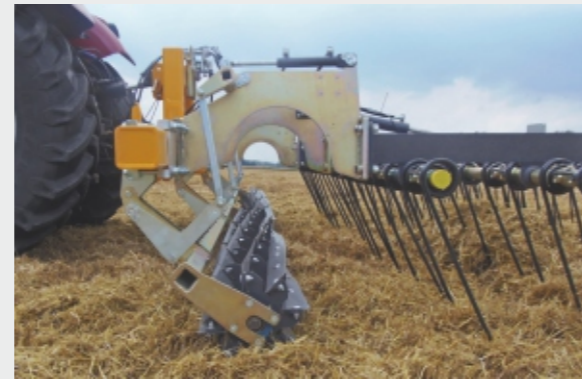
...also available with a Wallner harrow/knife roller.
