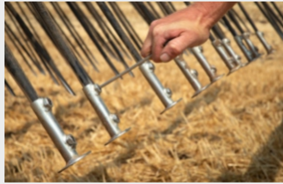
"Harrow Scratcher" cutting disks as teeth attachments - better cutting effect, e.g. for seedbed preparation in spring.
