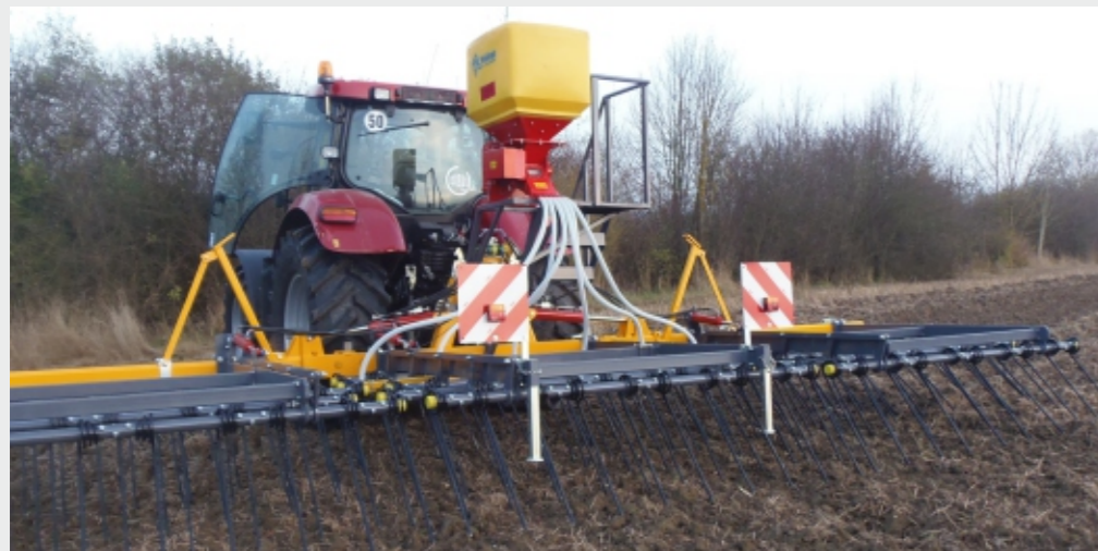
Standard with check valves on double-locking hydraulic cylinders. Optional protective cover for the teeth when driving on public roads.
