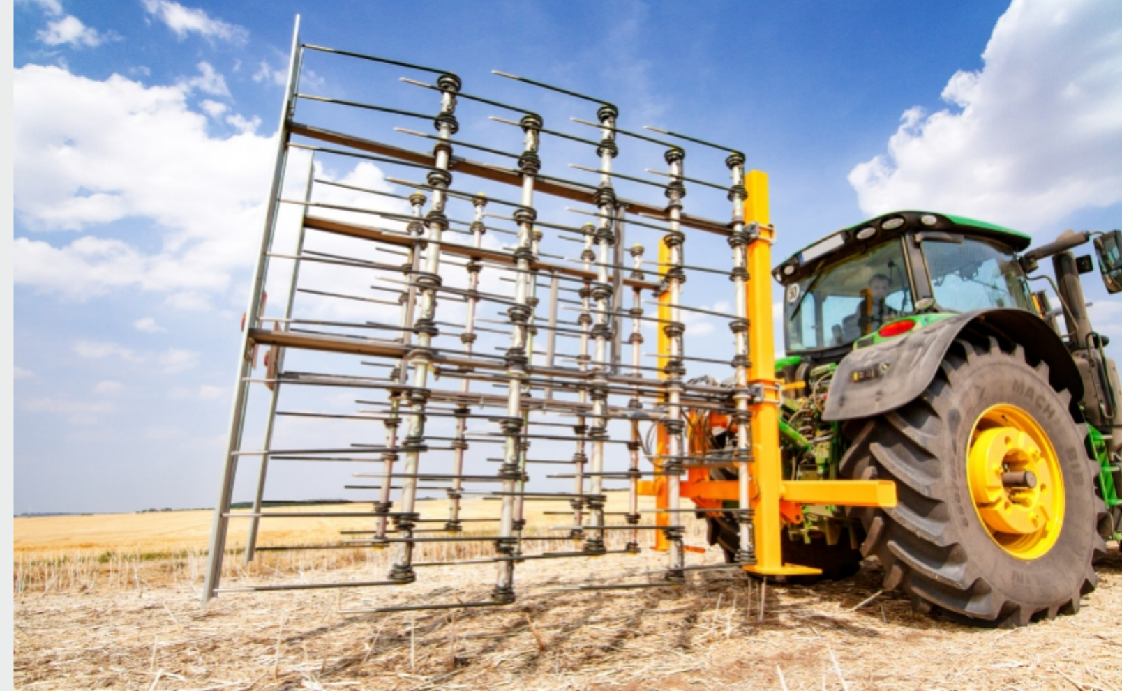
Additional option: "Harrow Carrier", for shallow scouring as an attachment to the harrow teeth - the teeth can be adjusted from deep plunging to light scouring.
